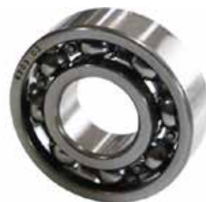
REF: 4024012 RODAMIENTO CAJA (6203 2RS C3) - (40 x 17 x 12)
